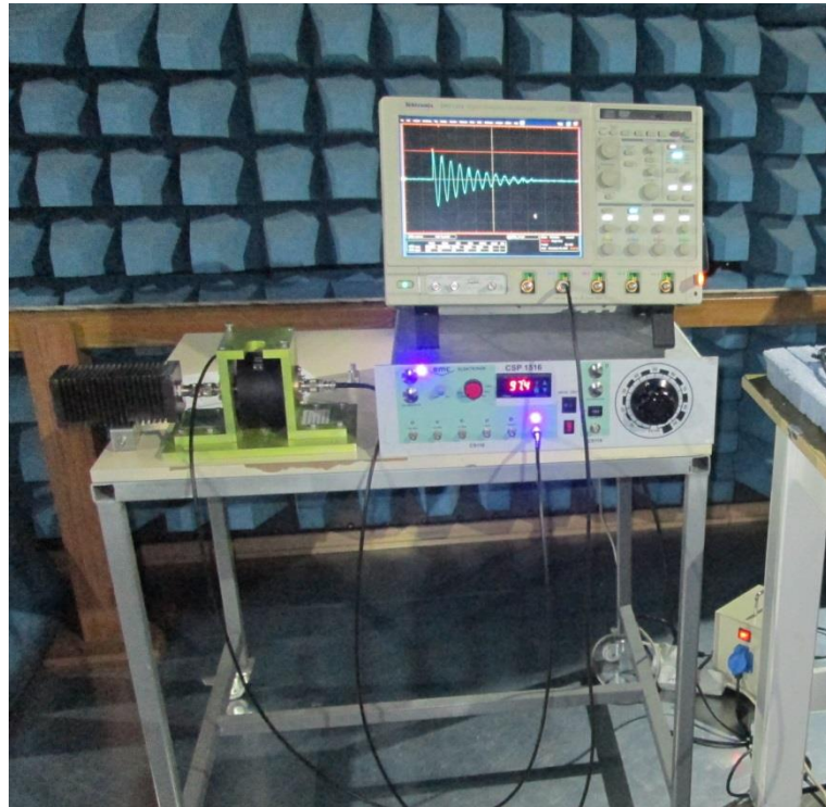
FIGURE A-17. Typical CS115 calibration fixture waveform.
